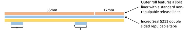
9mm strip of IncrediSeal 5211 double sided repulpable tape gets applied to a 100% repulpable release liner.
